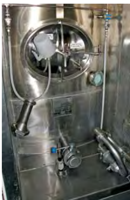
Easy access manway for cleaning and maintenance
